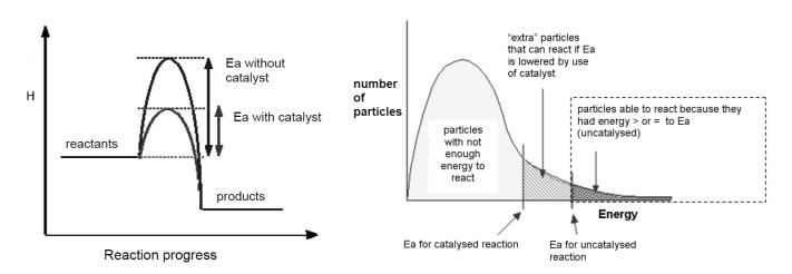
Be very careful if you are asked about how catalysts increase the rate of reaction in an examination. "A catalyst provides an alternative reaction pathway for the reaction with a lower activation energy."
